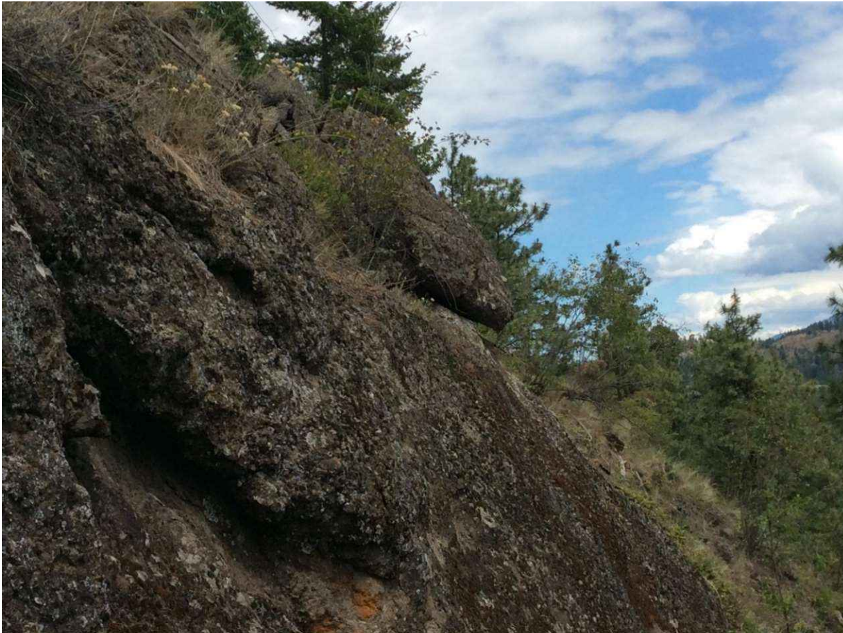
Photo 5.1b: Detached boulders and jointing were identified on bedrock exposures on the west slope above the 'mound' identified on the south end of the site. (Placemark 9, 2021-06-09)
